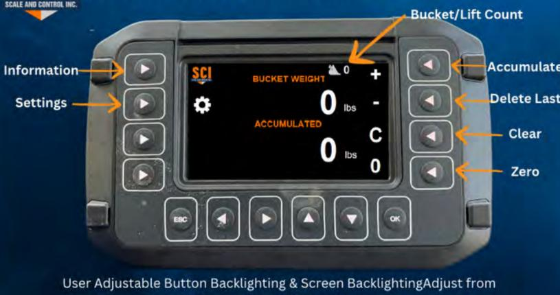
Iser Adjustable Button Backlighting & Screen BacklightingAdjust from 10% to 100%-In 10% Increments. Select Weight Units: LBS-KG-Tons-Tonnes
